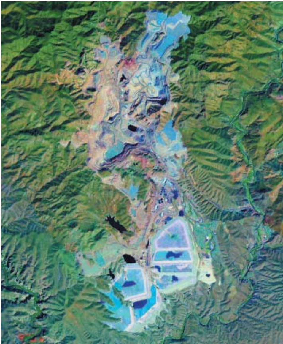
Morenci Open Pit mine, Greenlee County, Arizona: Landsat 7 false color image taken in October 1999 from an altitude of 438 miles. This image uses Thematic Mapper bands 1 (blue light), 4 (near-infrared light), and 7 (mid-infrared light). The area shown is 28 miles east-west and 39 miles north-south; visual resolution is 15 meters. Mine roads and benches can be seen in the tan-colored open pit, and tailings are visible as light blue areas. The town of Clifton is at center right, along the valley of the San Francisco River. Surface water is recognizable as dark blue or black areas. Image processed and enhanced by Kevin Horstman, copyright 2002.
