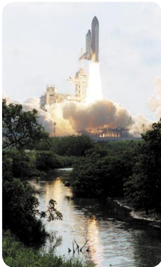
Space Shuttle Endeavor lifts off from the Kennedy Space Center, June 5, 2002. The large clouds produced upon launch result from the "burning" of approximately 385 tons of the oxidizer, ammonium perchlorate, in each of the two solid rocket boosters. Photo by NASA.
