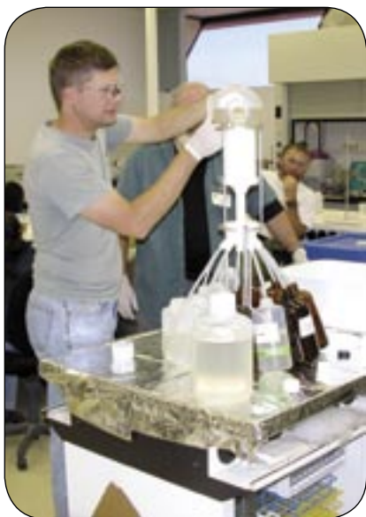
Tucson USGS employee Dave Anning uses a Teflon conesplitter to divide samples among 10 bottles to go to different labs for analysis.
