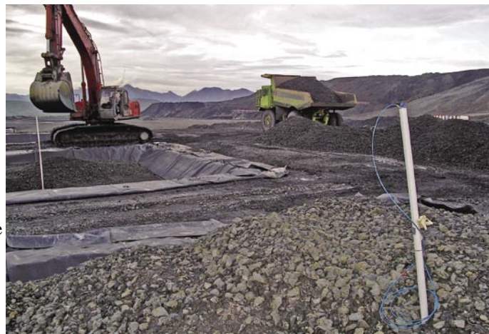
Placement of waste rock in test pits at Red Dog Mine, Alaska. A loaded and treated pit in the foreground shows wire leads from a thermistor placed in a vertical pipe for temperature measurements.
