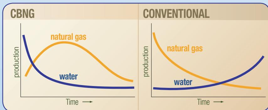
In coalbed natural gas production (left), water production is greatest at the beginning of operations. In contrast, water production increases with time in conventional oil and gas production (right).
