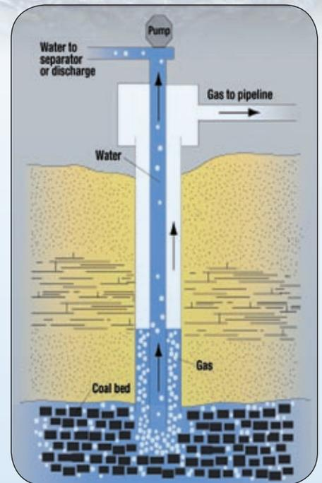
Diagram illustrating the production of water and gas in a typical coal-bed methane well. Source: USGS, 2004.
