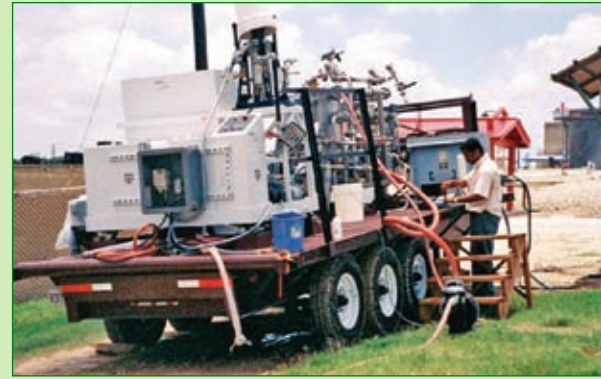
A&M's portable desalination unit at the old McFaddin Mercantile store near the site of the field pilot test.
